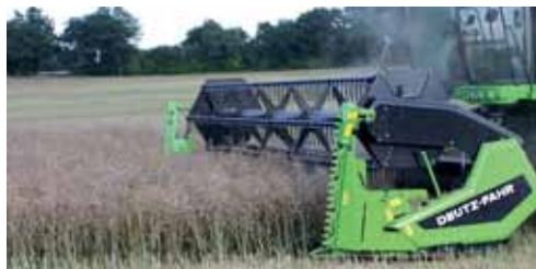
The rapeseed kit may be fitted to the grain header for even greater versatility.
