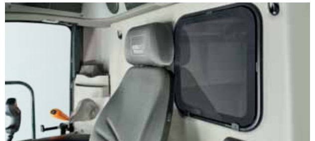
VISUAL GRAIN TANK MONITORING. A window in the cab lets the operator visually check the fill level of the tank and the quality of the grain harvested.
