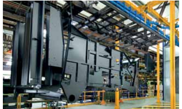
All the painted parts of the machine are treated with an advanced cataphoresis process in which each individual part is immersed in a series of 14 different tanks, starting with a cleaning treatment and polarisation, and concluding with the paint process.
