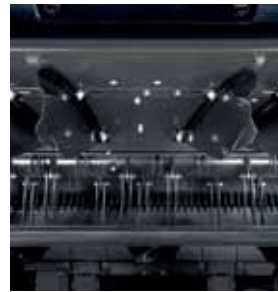
STRAW CHOPPER. For even more effective material distribution, the straw chopper may also be equipped with deflectors, adjusted electrically from the cab, to adjust spreading to weather conditions.
