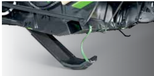
The sensor skids allow the header to follow the contours of the terrain precisely and make instant adjustments to ensure an even cutting height.
