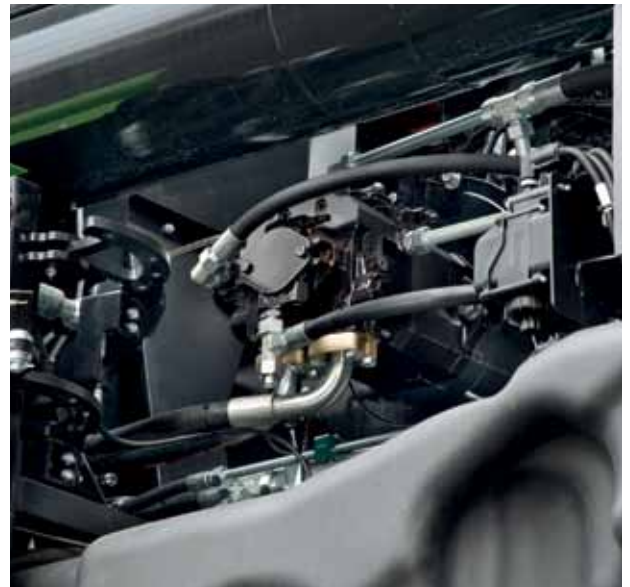
VARIABLE DISPLACEMENT PUMP. The hydrostatic pump is fitted directly to the engine.
