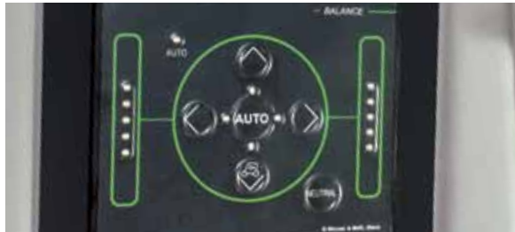
The Balance system adjusts the position of the entire machine completely automatically to correct for lateral gradients up to 20% and longitudinal gradients up to 6% and keep the combine harvester perfectly level.
