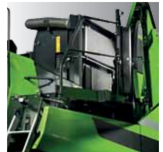
ACCESS FOR RADIATOR CLEANING.
