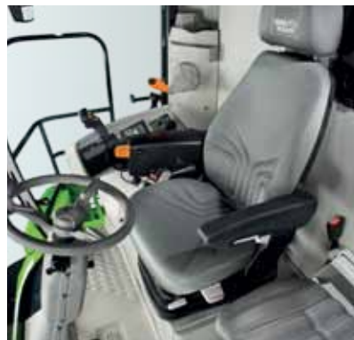
Ergonomic seat with mechanical or pneumatic adjustment and adjustable steering column for setting the a comfortable driving position.
